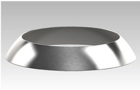
One of the family of 17 parts that nest together for oil drilling. 35" to 40" DIAMETER X 4.00" to 6.00" Height X 0.250" thick 304 s/s. Parts are spun on a CNC spinning lathe.
