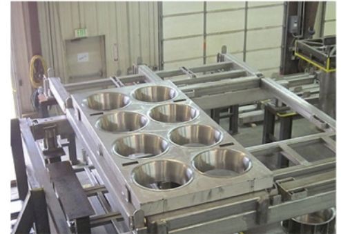
Customer picture of assembly for waste storage project using flanged cones spun at Helander Metal Spinning Company.
